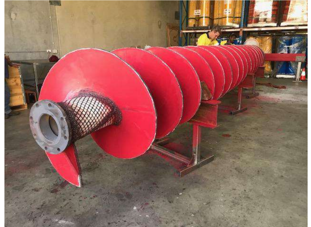
👉 Lithium Screw feeder improvement (rubber & ceramic lining work)
