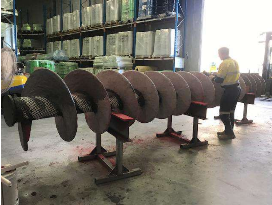
👉 Lithium Screw feeder improvement (rubber & ceramic lining work)
